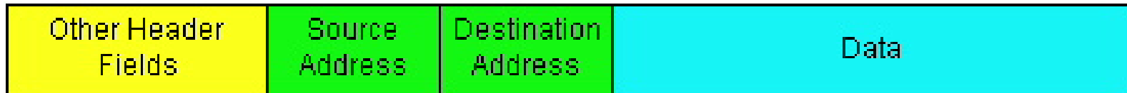
Figure 4.4-5: The key fields in an IP datagram.
