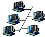
shared wire (e.g., cabled Ethernet)
