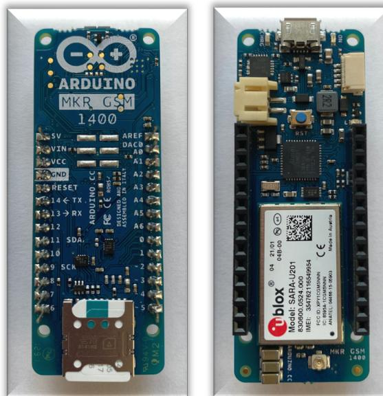
Figure 2-1 - Arduino MKR GSM 1400
