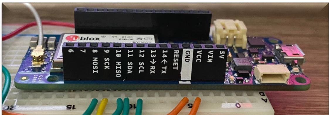
Figure 2-6 - SPI communication connections
