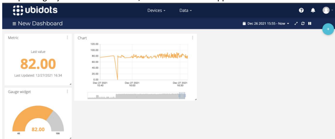
Figure 8 variables in dashboard, live reading from the ESP8266
