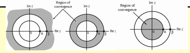
• In general, the ROC  $\mathcal{R}$  of a z-transform of a sequence g[n] is an annular region of the z-plane:
