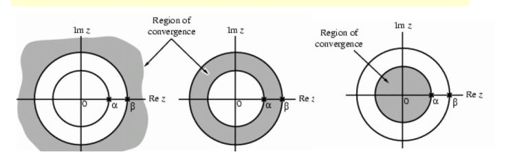
The ROC of a rational z-transform can be easily determined using MATLAB
