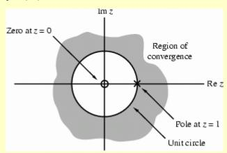
• In this plot, the ROC, shown as the shaded area, is the region of the z-plane just outside the circle centered at the origin and going through the pole at z = 1
