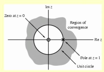
• A physical interpretation of the concepts of poles and zeros can be given by plotting the log-magnitude  $20\log_{10}|G(z)|$  as shown on next slide for
