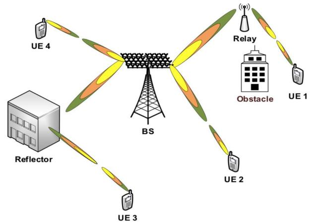
Employing adaptive **beamforming** to suppress interference
