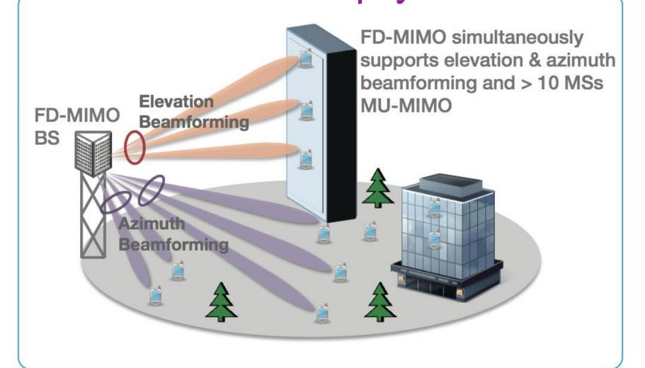
Large Scale Antenna Systems (LSAS), Full Dimension MIMO (FD-MIMO), Very Large MIMO , Hyper MIMO.
