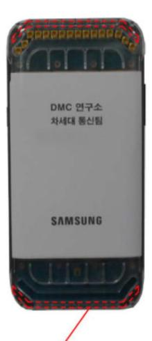
16-antenna arrays at the top and bottom of a prototype Samsung phone CREDIT: SAMSUNG
