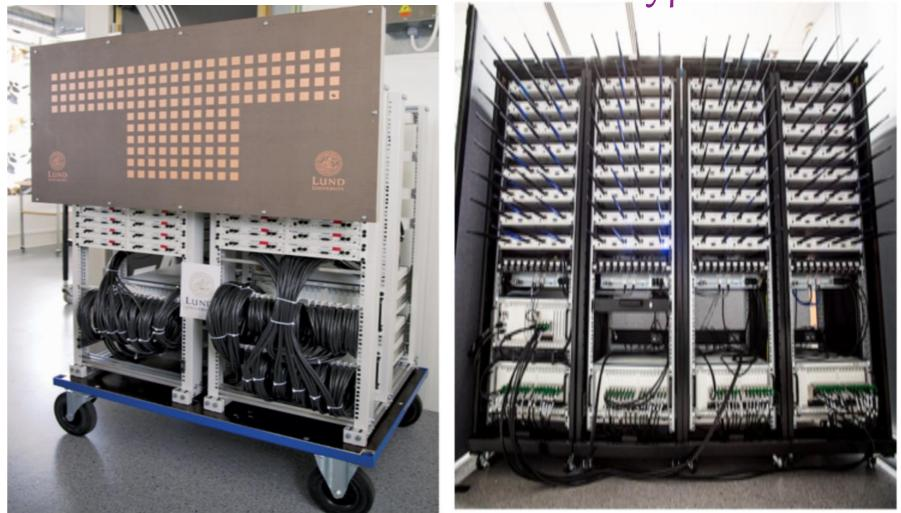
Lund University / NTT Docomo massive MIMO prototype Up to 1024 and 64 for the BSs and UEs, respectively. (with <u>RF chains</u>, the maximum numbers are 32 and 8 for the BSs and UEs) Evolution of Multi-antenna Technology From 4G MIMO to 5G Massive MIMO
