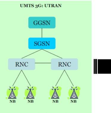
NB: NodeB (base station) RNC: Radio Network Controller SGSN: Serving GPRS Support Node GGSN: Gateway GPRS Support Node
