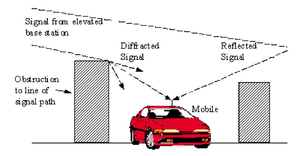
Figure 2 Radio Propagation Effects
