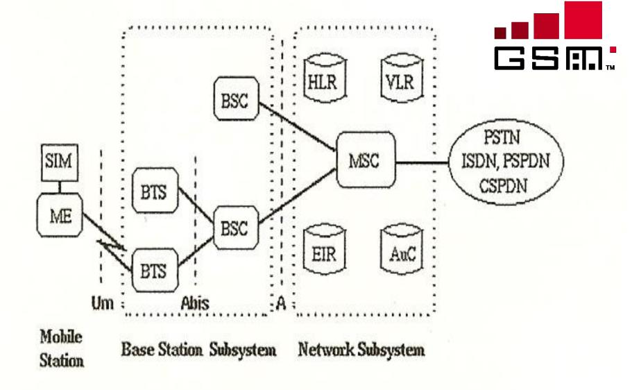
SIM Subscriber Identity Module ME Mobile Equipment BTS Base Transceiver Station BSC Base Station Controller HLR Home Location Register VLR Visitor Location Register
