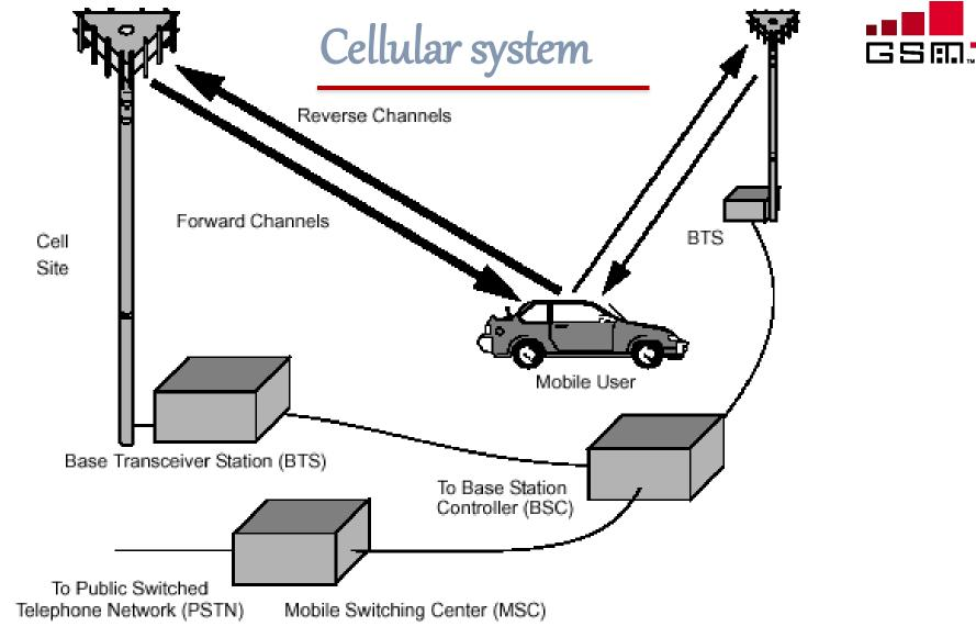
Figure 1–3 There are two main types of forward channels. Control and access channels are used to set up calls and provide security and management functions. Traffic channels are used to carry voice traffic. The reverse channels are also divided into access channels and traffic channels. In some systems, the Base Station Controller (BSC) may be integrated directly into the cell site. In other systems, as shown here, the Base Transceiver Stations (BTSs) are connected to a Base Station Controller.
