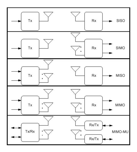
SISO: Single input Single output SIMO: Single input Multiple output MISO: Multiple input Single output MIMO: Multiple input Multiple output MIMO-MU: Multiple input Multiple output (multiuse By: Dr.Mohab Mangoud
