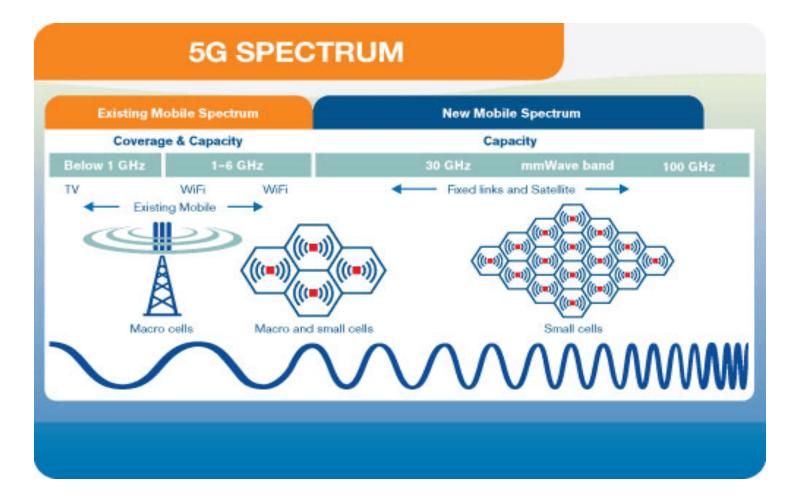
5G will use spectrum: 600 MHz to 6 GHz + mmWave bands (24–86 GHz).
