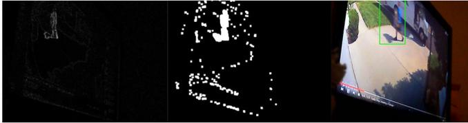
Fig. 8. Demonstration for the process that the motion detection code goes through to detect the motion, while its starting from the left side where that process the image to grey colors. The middle image is after applying the blur, threshold, and dilated codes. Finally, it compares the contours and draws the green rectangle on the detected motion.
